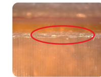
Edge of solid is damaged from excessive Anilox impression
