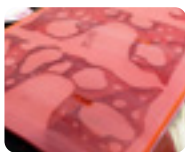
This is what Solvent Entrapment looks like between two plates
