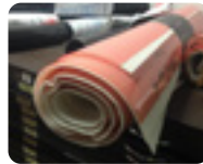
Plate should be rolled face outward with foam to reduce plate lift on press
